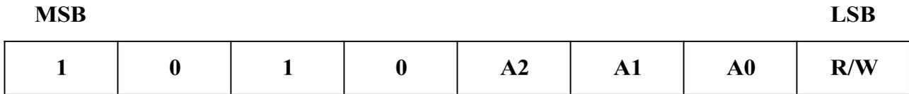
**Figure 5. Device Address**
