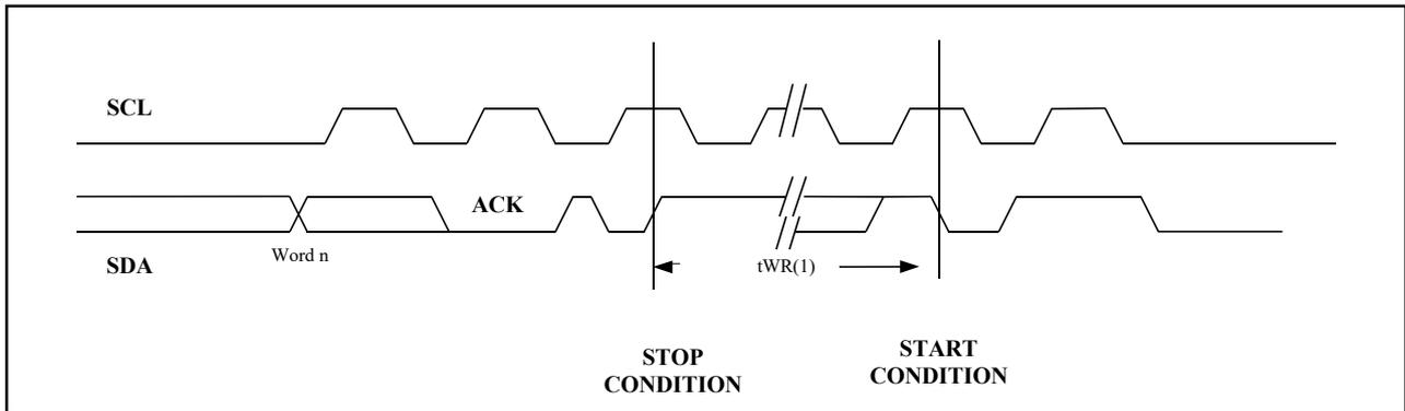
**Figure 12. SCL: Serial Clock, SDA: Serial Data I/O**
