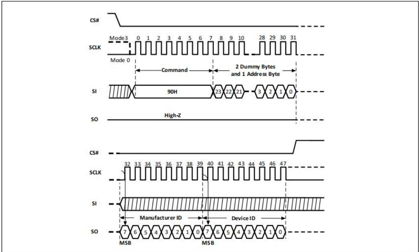
**4.30 Dual I/O Read Electronic Manufacturer ID & Device ID (DREMS) (92H)**
