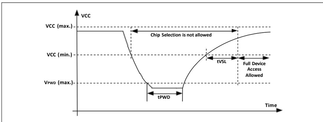
**Table-17 Power-Up Timing and Write Inhibit Threshold**
