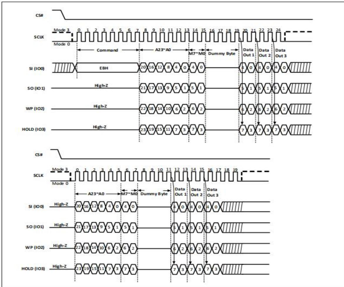
**Note:** Quad I/O Fast Read with “Continuous Read Mode”, if (M5-4)=(1,0). If not using “Continuous Read Mode” recommend setting (M5-4)≠(1,0).
