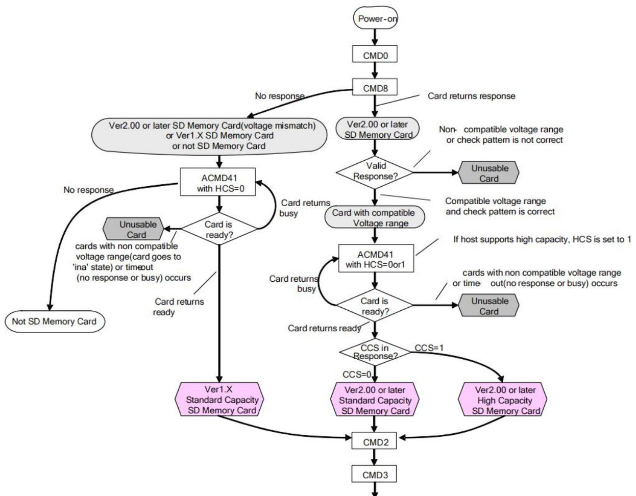
**Figure 6.2.1: Card Initialization and Identification Flow (SD mode)**
