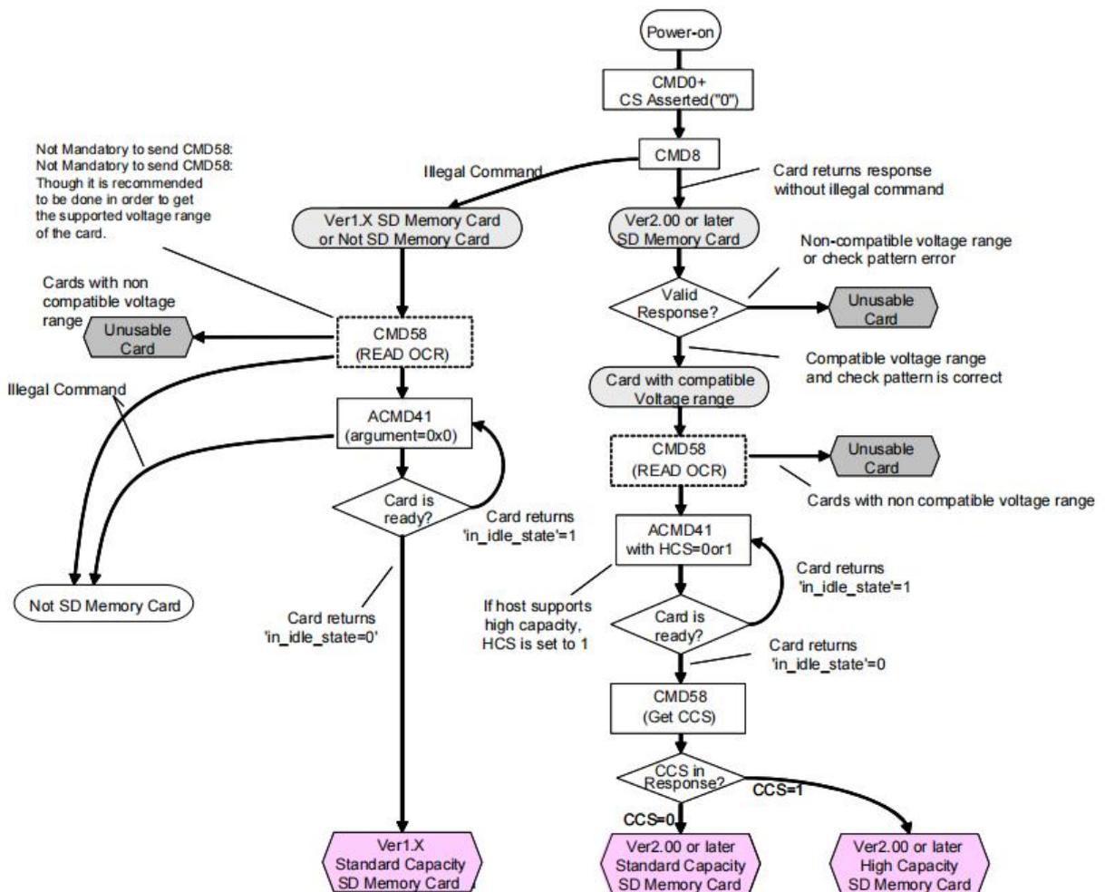
Figure 6.2.2: SPI Mode Initialization Flow
