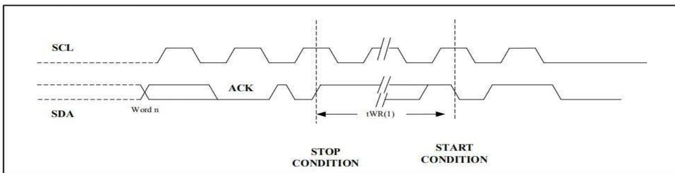
Figure 12. SCL: Serial Clock, SDA: Serial Data I/O
