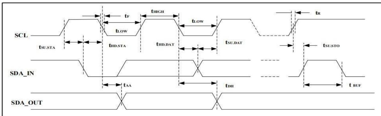
Figure 11. SCL: Serial Clock, SDA: Serial Data I/O
